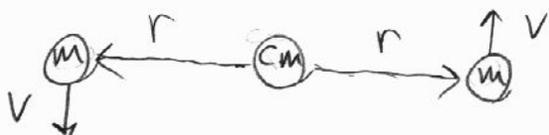
$$\text{KE: } U_k = 2 \times \frac{1}{2} m v^2 = m v^2$$
