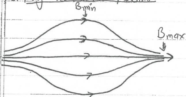
1. Particles are confined by magnetic mirror force at either end of the machine.
