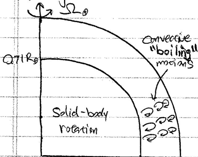
1. Motions of the solar plasma with the convection zone at  $r \geq 0.71 R_{\odot}$  support the solar magnetic dynamo
