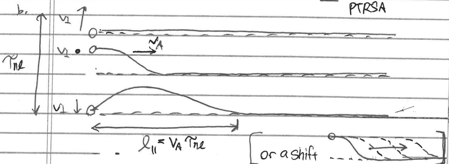
c. Now,  $\ell_{\parallel} = v_A \left( \frac{\ell_{\perp}}{v_{\perp}} \right) \Rightarrow \frac{\ell_{\parallel} v_{\perp}}{\ell_{\perp} v_A} = 1 \Rightarrow \frac{k_{\perp} v_{\perp}}{k_{\parallel} v_A} = \alpha = 1$
