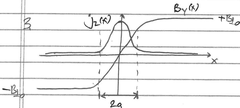
4. Pressure Balance: Note that in equilibrium, the Harris Sheet requires a pressure variation  $p_0(x)$  to balance magnetic pressure along  $x$ ,  $\frac{2}{x} (p_0(t) + \frac{(B_0)^2}{2\mu_0}) = 0$ .
