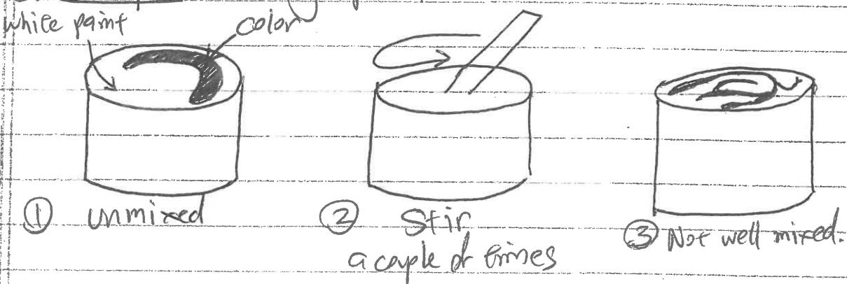
⇒ The difference in results is due to turbulence!
