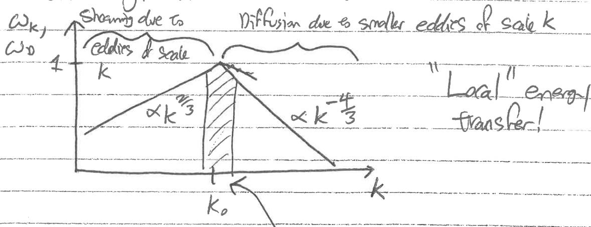
a. The peak occurs at  $k \approx k_0$ . Thus, it is the shearing/diffusion due to the local scale eddies with  $k \approx k_0$  that dominates energy transfer from eddies at  $k_0$  to smaller scales/higher wavenumbers, i.e.  $k_0 \rightarrow 2k_0$ .
