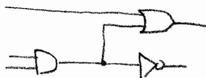
OK: two inputs connected to one output
