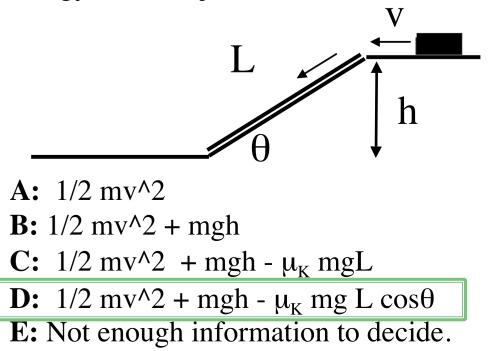
FF = MN Mg (os of = mmg (os of  $E_{o} = mgh + y_2 mv^2$ = E. + Winc E,  $= E_{e} - F_{F} - L$ = Eo - pring cost & L = mgh + 12mv2 - µmg cosol
