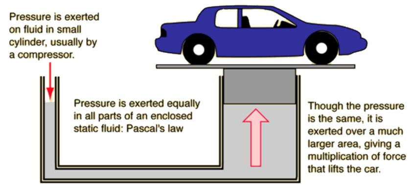
The force in the small cylinder must be exerted over a much larger distance. A small force exerted over a large distance is traded for a large force over a small distance.
