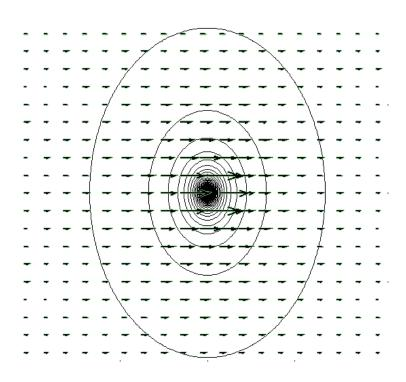
E = - DV - AAST B = DXA In general -Out R A depend on F t so messy to calculate even for special case of const. velocity - LOOK 6) A = 0  $\times > Vt$   $V(x,t) = \frac{\alpha}{4\pi \epsilon_0 R} = \frac{\alpha}{4\pi \epsilon_0 |\vec{r} - \vec{v}t|}$ 411E0 (X-V+) A(x/t) = ZV 4120C2 (X-V+) = 9x -V 4TG. (x-v+)2 + 9vx -V 4TEOC2 (x-v+)2 41/2 (1-V2)
