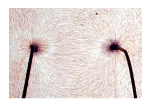
Torque on little dipoles (felt fibers) aligns them with the electric field
