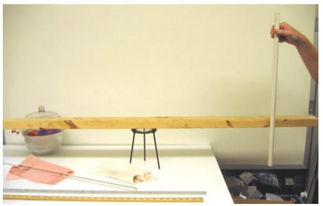
Force on little dipoles (molecules in wood) from diverging electric field of charged object pulls them toward the charge
